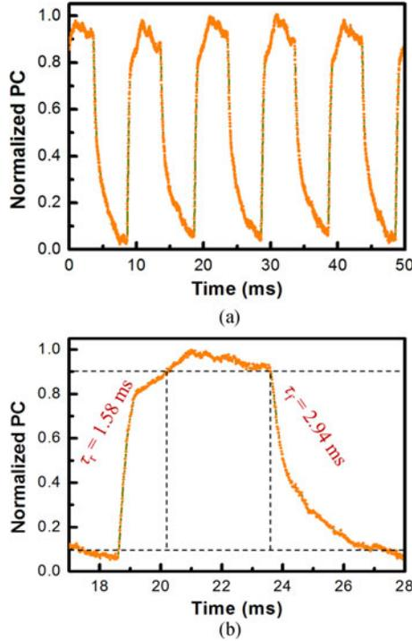
Fig. 7. (a) Normalized photocurrent versus time under 100 Hz 1550 nm illumination at  $V_{gs} = 30$  V and  $V_{ds} = 1$  V. (b) The enlarged picture to show detailed rise time ( $\tau_r$ ) and fall time ( $\tau_f$ ) of the hybrid phototransistor.
