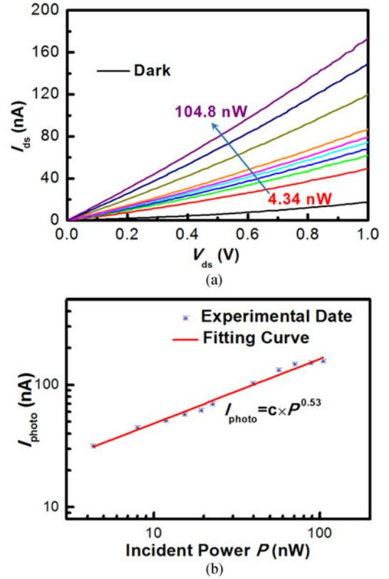
Fig. 5. (a) Linear  $I_{ds}$  versus  $V_{ds}$  curves under 1550 nm illumination with different illumination power intensities varied from 4.34 nW to 104.8 nW at  $V_{ds} = 1$  V and  $V_{gs} = 30$  V. (b) Dependence of photocurrent on illumination power intensities.
