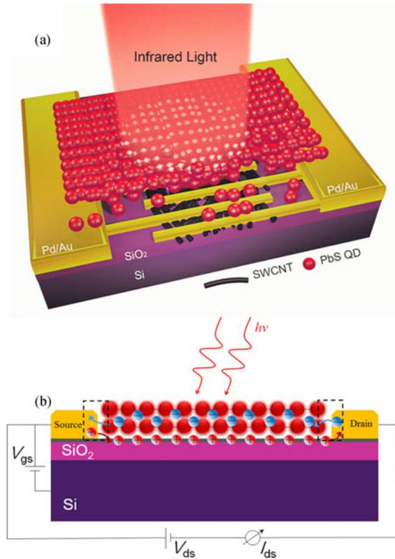
Fig. 1. (a) Three-dimensional schematic of the SWCNT film-PbS QDs hybrid phototransistor with interdigital finger electrodes. (b) Schematic of the photo-response circuit of the device showing the voltage bias.  $V_{ds}$ , source–drain voltage;  $V_{gs}$ , gate–source voltage.
