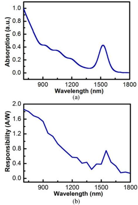
Fig. 3. (a) Normalized absorption spectra of the PbS QDs. (b) Normalized spectral responsivity of the hybrid phototransistor with  $V_{gs} = 30$  V and  $V_{ds} = 1$  V.
