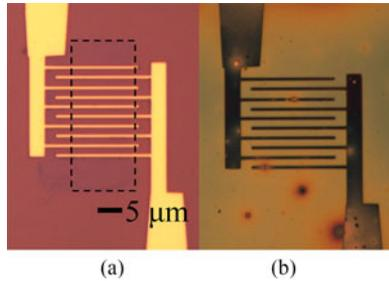
Fig. 8. (a) Optical image of the etched SWCNTs film with interdigital finger electrodes, where the dark dotted box shows the film edges. (b) Optical image of the device after the LBL spin-coating process of PbS QDs.
