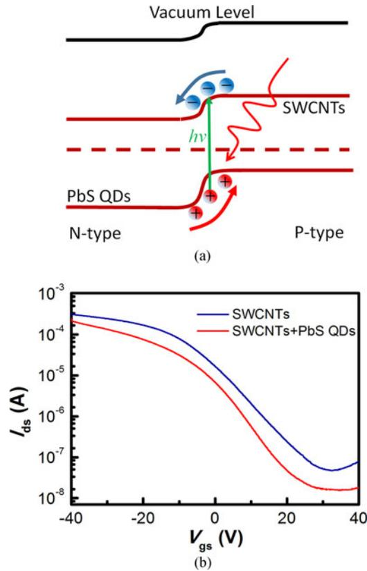
Fig. 2. (a) Schematic of band diagram for built-in electric field assisted charge transfer between PbS QDs and SWCNTs under illumination. (b) Transfer characteristics of SWCNTs film only and PbS QDs/SWCNTs hybrid structure with  $V_{ds} = 1$  V.
