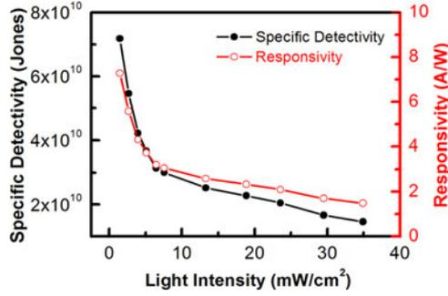
Fig. 6. Specific detectivity and responsivity of the hybrid phototransistor at  $V_{ds} = 1$  V and  $V_{gs} = 30$  V.
