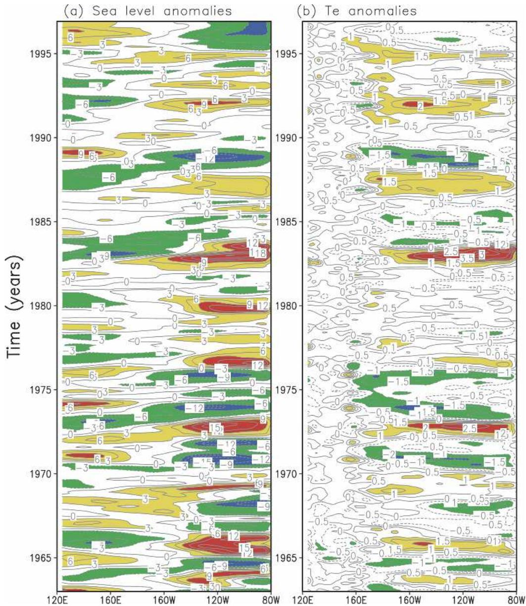
FIG. 2. Anomalies along the equator during the period 1963–96 of sea level (a) simulated from an intermediate dynamic ocean model and (b)  $T_e$  estimated from the inverse modeling. The contour interval is 3 cm in (a) and 0.5°C in (b).
