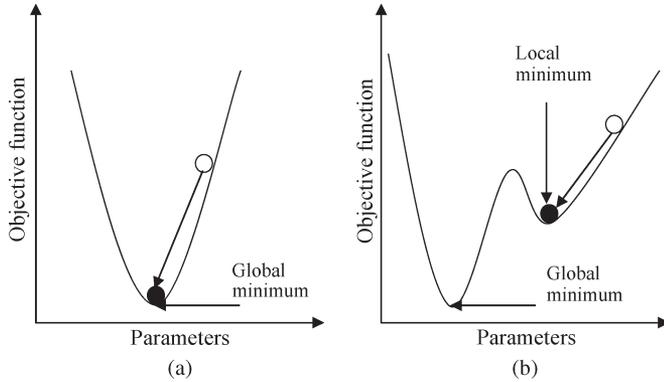
Fig. 1. Objective functions of the parameters of (a) SVR and (b) conventional nonlinear least squares regression and ANN.
