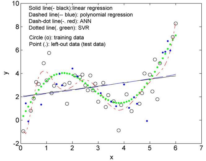
Fig. 4. Functions developed by four regression methods on one training data set.
