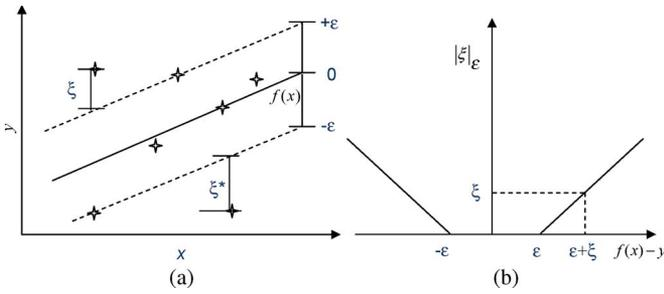
Fig. 2. (a) Loss setting for linear SVR and (b)  $\varepsilon$ -insensitive loss function.
