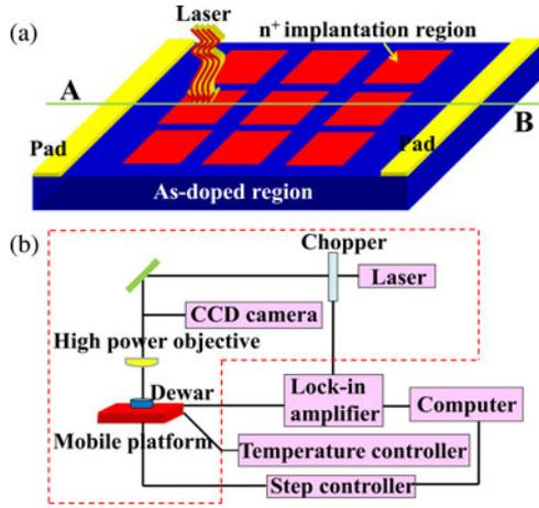
Fig. 1. (a) Schematic of HgCdTe infrared detector pixel arrays. The pixel size of the detector pixel array is  $200 \mu\text{m}$  with the array format of  $256 \times 256$  pixels. The ion-implantation window is  $50 \mu\text{m} \times 50 \mu\text{m}$ . (b) Experimental setup for measurement of laser beam induced current.
