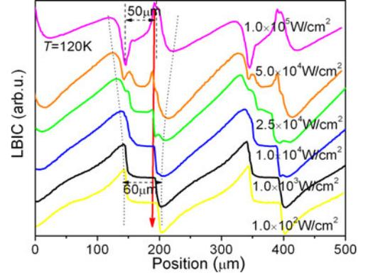
Fig. 2. Experimentally measured LBIC signal profiles (a) at a temperature of 120 K with the laser irradiances of  $1.0 \times 10^2$ – $1.0 \times 10^5$  W/cm<sup>2</sup>. The illumination laser wavelength is 0.63  $\mu$ m.
