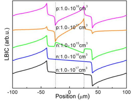
Fig. 7. Numerical simulations of the LBICs based on the proposed model in Fig. 5(a) with the different doping densities and doping types in the ion implantation region.
