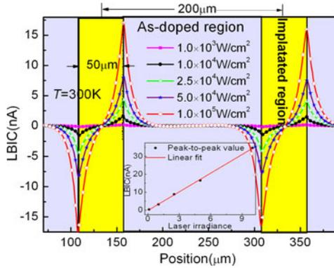
Fig. 4. Experimentally measured laser-irradiance-dependent LBIC signal profiles at a temperature of 300 K. The inset shows the peak-to-peak value of LBIC at different laser irradiances.
