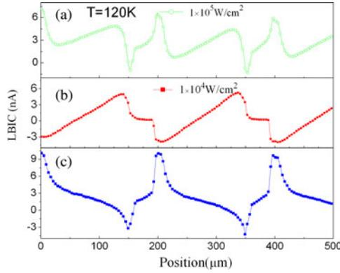
Fig. 3. Experimentally measured LBIC signal profiles (a) at a laser irradiance of  $1 \times 10^5$  W/cm<sup>2</sup> and (b) at a laser irradiance of  $1 \times 10^4$  W/cm<sup>2</sup>. (c) Net LBIC value by subtracting the  $y$ -axis value of (a) with the  $y$ -axis value of (b). The temperature for all the measurements is 120 K.
