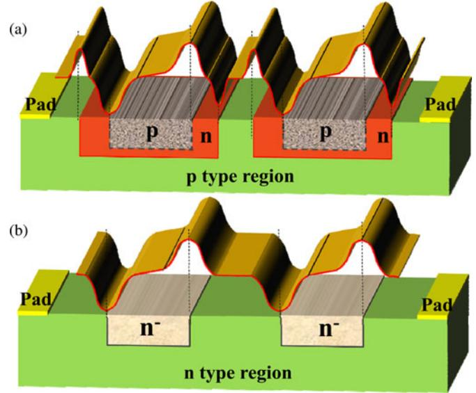
Fig. 5. Schematic of proposed ion-implantation-induced junction transformation models. (a) The p-n-on-p junction is formed at low temperature and high laser irradiance, where the photo-generated carriers are the large injection compared to temperature-induced carriers. (b) The p-on-n junction is formed at room temperature and low laser irradiance, where the photo-generated carriers are the low-level injection compared to temperature-induced carriers.
