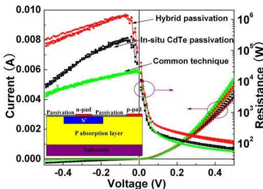
FIG. 2. (Color online) Measured dynamic resistance (right axis) and dark current (left axis) with different surface passivation techniques.
