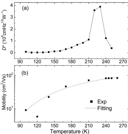
FIG. 2. (a) Temperature dependence detectivity with chopping frequency of 1000 Hz. (b) Drift mobility versus temperature for experiment (closed square) and theoretical result (dash line by fitting Eq. (1)).
