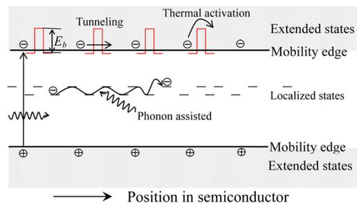
FIG. 4. (Color online) Electric conduction mechanisms are illustrated schematically for the electrons. Similar processes are also suitable for the holes.
