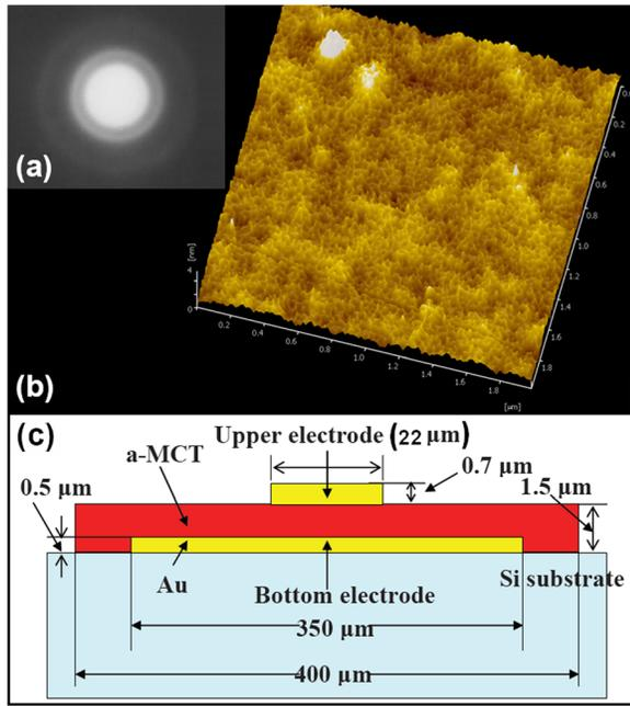
FIG. 1. (Color online) (a) Electron diffraction pattern and (b) AFM surface morphology of a-MCT film. (c) Schematic diagram of a-MCT infrared photoconductive detector structure.
