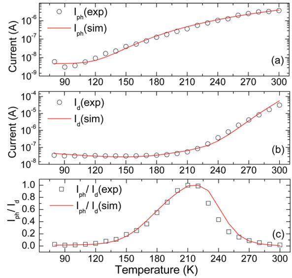
FIG. 3. (Color online) Comparisons of the experimental and calculated currents vs temperature at bias of 9.0 V. (a)  $I_{ph}$  and (b)  $I_d$  with the hollow circles and solid lines being the experimental and calculated results, respectively. The  $I_{ph}/I_d$  at different temperature is shown in (c). The hollow squares represent the measured values, and the solid line is the results of numerical calculations.
