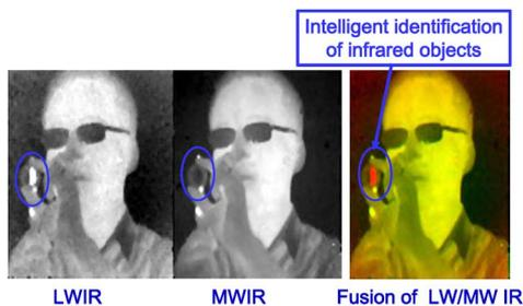
Fig. 6. Infrared image from the  $128 \times 128$  LW/MW HgCdTe two-color infrared FPA detector at 77 K. A MW optical filter is used to stop MW infrared radiation. The heated electric soldering iron behind the filter is invisible for the MWIR detector (middle) while visible for the LWIR detector (left).
