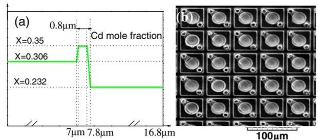
Fig. 4. (a) Designed Cd mole fraction of  $p_1$ , P, and  $p_2$  layers during the HgCdTe material epitaxial growth. (b) SEM image of the  $128 \times 128$  LW/MW HgCdTe two-color infrared FPA detector.
