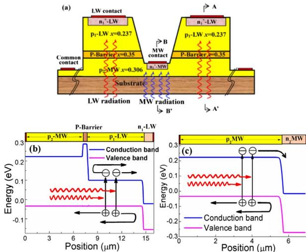
Fig. 1. (a) Schematic of grooved HgCdTe two-color infrared detector. (b) Equilibrium energy band diagram cut at A - A'. (c) Equilibrium energy band diagram cut at B - B'.
