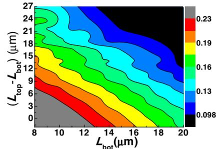
Fig. 3. LW QE as functions of  $(L_{\text{top}} - L_{\text{bot}})$  and  $L_{\text{bot}}$  at a LW cutoff wavelength of 9.7  $\mu\text{m}$ .
