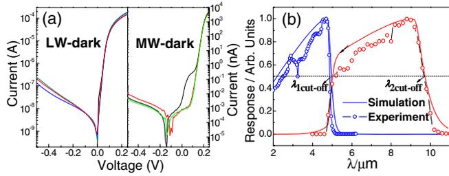
Fig. 5. (a) Dark current characteristics of LW and MW junctions. (b) Experimental (dotted) and simulated (solid) spectral photoresponse of the LW/MW HgCdTe two-color infrared detector with cutoff wavelengths of  $\lambda_{1 \text{ cut-off}} = 4.8 \mu\text{m}$  and  $\lambda_{2 \text{ cut-off}} = 9.7 \mu\text{m}$  for the LW and MW diodes, respectively. A voltage of 0.01 V is used in the simulation and experiment.
