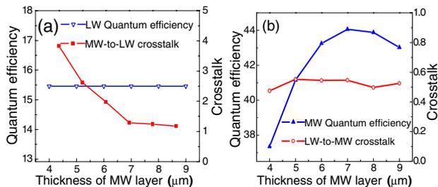
Fig. 2. (a) LW QE and MW-to-LW cross talk and (b) MW QE and LW-to-MW cross talk as a function of the thickness of the MW layer for the infrared detector. The QE is calculated at the cutoff wavelength.
