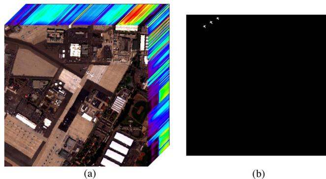
Fig. 3. AVIRIS data set and the distribution of the targets. (a) Hyperspectral cube of the San Diego image; (b) The true locations of the targets.
