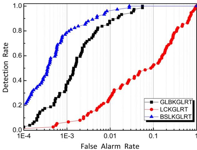
Fig. 7. The ROC curves of GLBKGLRT, LCKGLRT, and BSLKGLRT for the San Diego image.
