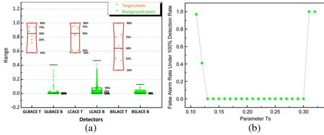
Fig. 4. (a) Target-background separation diagram for the RIT image. (b) Sensitivity analysis of parameter  $T_s$ .
