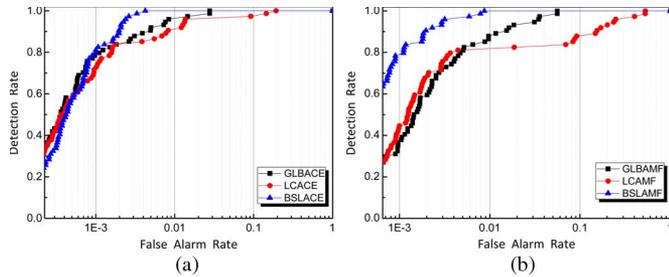
Fig. 6. (a) ROC curves of GLBACE, LCACE, and BSLACE for the San Diego image. (b) ROC curves of GLBAMF, LCAMF, and BSLAMF for the San Diego image.
