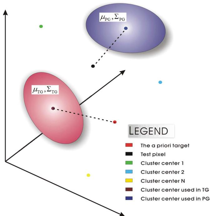
Fig. 1. Diagram illustrating how to properly assign clusters for the test pixels.
