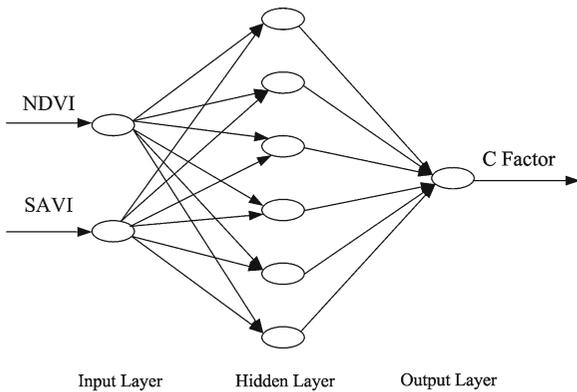
**Fig. 4** Structure of the BP neural network used for *C* factor evaluation
