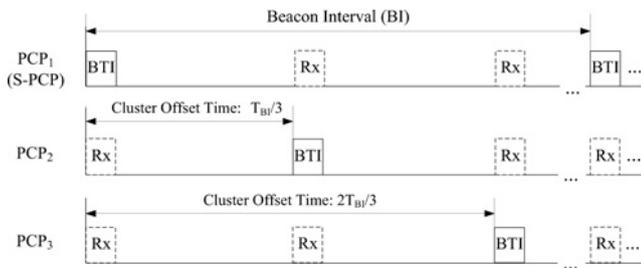
Fig. 2 Example of cluster mechanism (three PCPs in a cluster)
