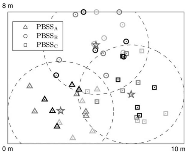
**Fig. 7** Simulated network in a cubicle room (three random cases: distribution of each case is depicted by markers with black, grey and light grey edge respectively, and stars stand for PCPs in each PBSS)
