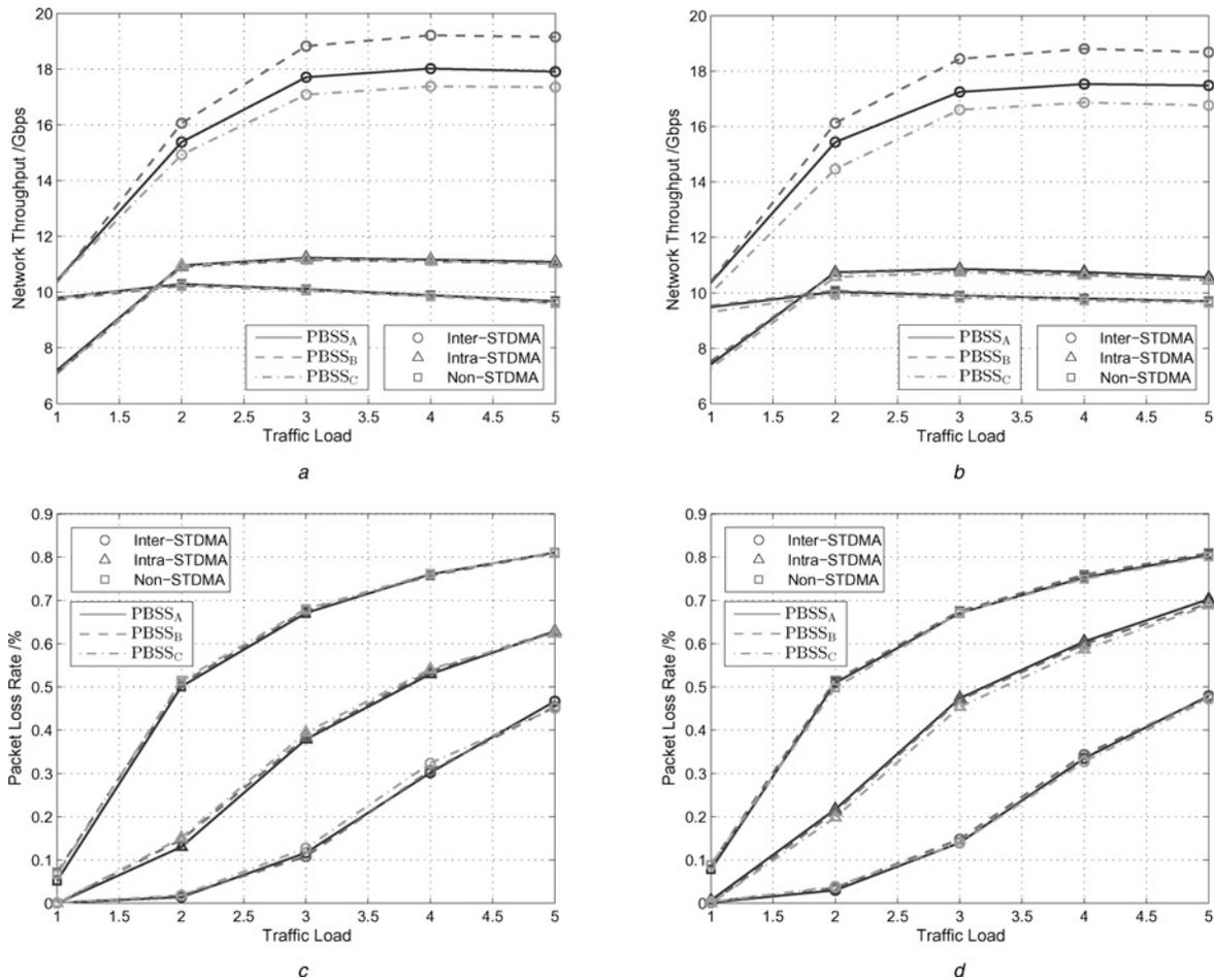
Fig. 8 Network throughput and average packet loss rate of three scheduling schemes under uniform and non-uniform Poisson patterns
