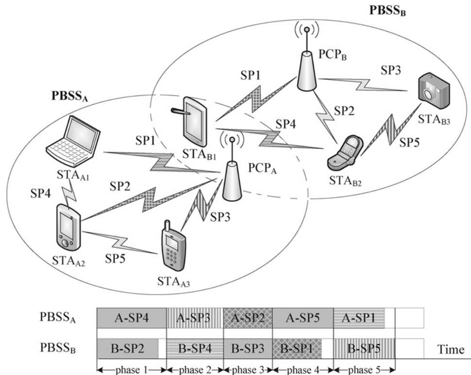
Fig. 3 System model: spatial reuse and interference mitigation among co-channel PBSSs
