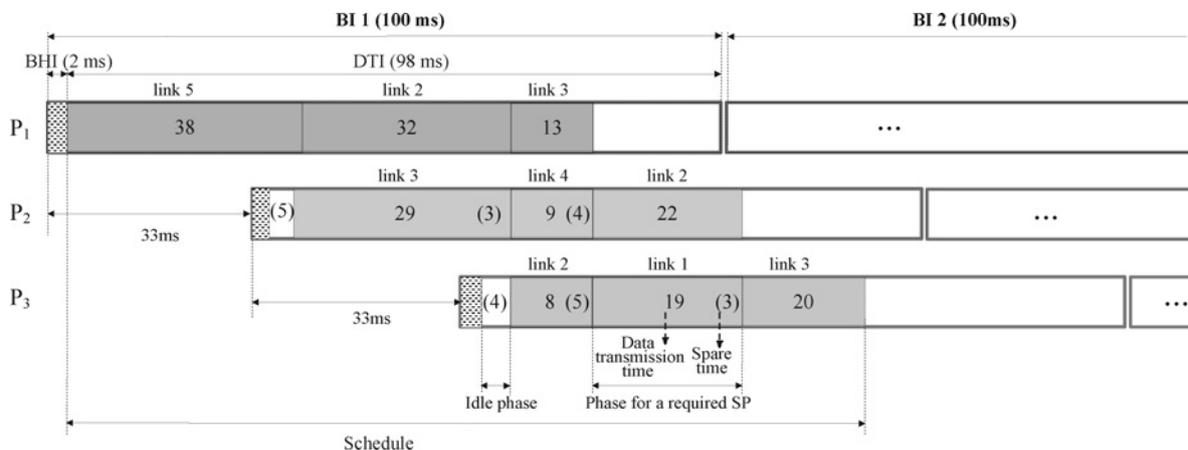
Fig. 6 Example of the first schedule of three co-channel PBSSs adopting STDMA scheduling algorithm
